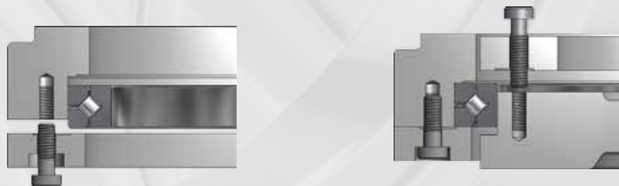
Mounting Crossed roller bearing with clamping rings
