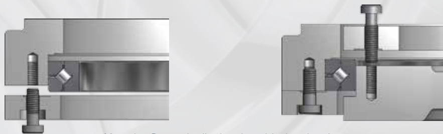
Mounting Crossed roller bearing with clamping rings
