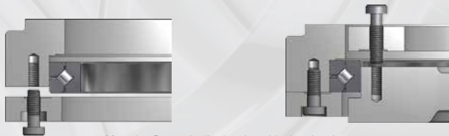
Mounting Crossed roller bearing with clamping rings
